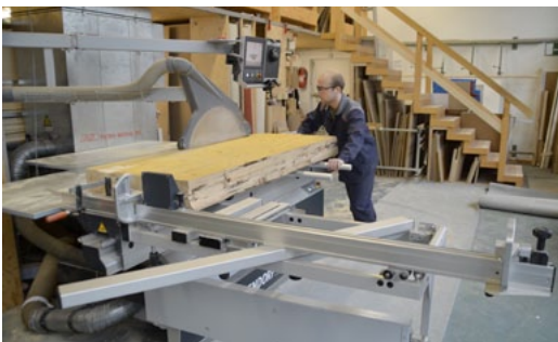
Sawing the former "Tivoli" beams to wooden floor boards
