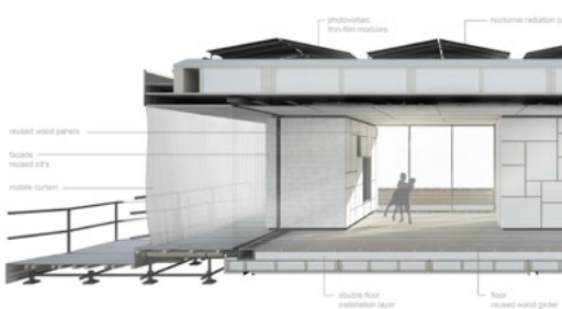
Section of the cantilevering roof and curtain
