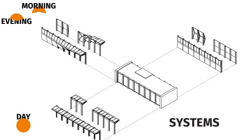
to keep things light we opt for an aluminium frame. The lifting movement is realised with two cable winchs inside rails fixed on the neighbouring wooden pillars. The lower wing's base is fixed on these cables, the motor's actuator force is translated into movement here. A shaft connects the motor to both rails. The upper wing is connected to the lower with a bolt, and to the house with a hinge at top. Why the engineering effort?
