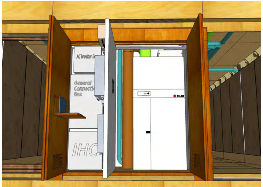
Fig 49. Technical Block View of electric panel with TB rear doors opened and electric panel opened giving way to NILAN VP18 maintenance front doors and control panel.
