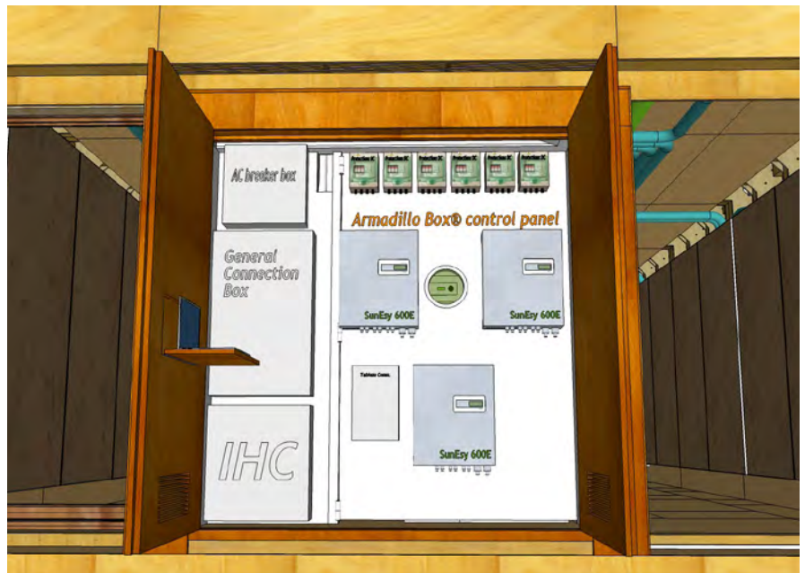
Fig 50. Technical Block View of electric panel with TB rear doors opened. Left reardoor contains a foldable table for laptop that can be connected to IHC in order to steer the installation.
