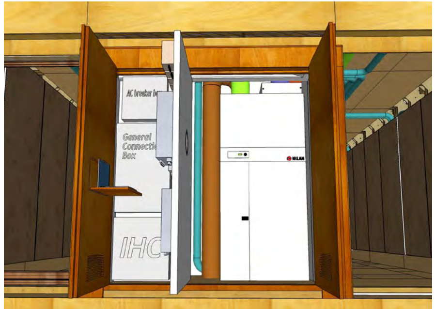
Fig 14. Technical Block View of electric panel with TB rear doors opened and electric panel opened giving way to NILAN VP18 maintenance front doors and control panel.
