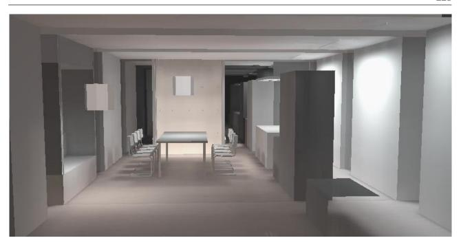
Figure 5: Simulation with Dialux of the artiticial light without gaps lighting
