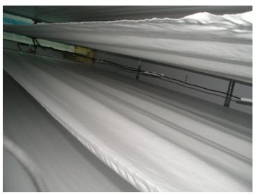
Figure 5: Experimental setup of the ventilation tower (textiles used as moist surfaces) [13].
