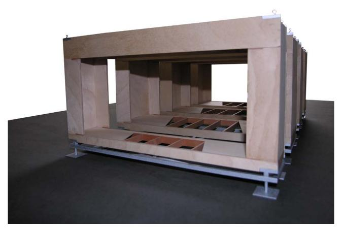
Figure 2: model of timber module
