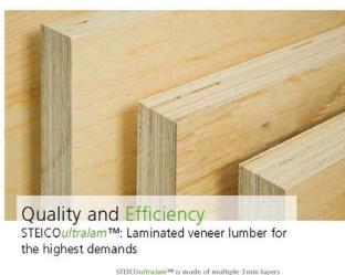
STEICOultralam<sup>TM</sup> is made of multiple 3 mm layers of graded laminated spruce veneers. This disperses knots and irregular growth, producing a practically homogeneous cross section. This construction means that STEICOultralam<sup>TM</sup> is highly rigid and dimensionally stable.
