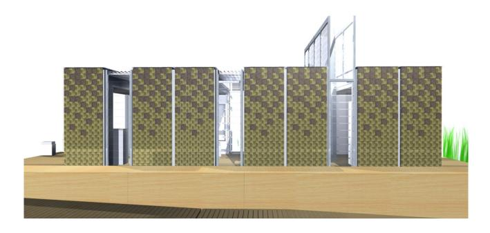
The modules are positioned with interspaces between them. These gaps are part of the design concept to point up the modularity. But the gaps are much more than only design. They are used for lighting, ventilation, pre-heating in winter and passive cooling in summer. They also allow for a visual connection to the outside and offer very different view axes withinthe building and to the outside by nicely framing the exterior.
