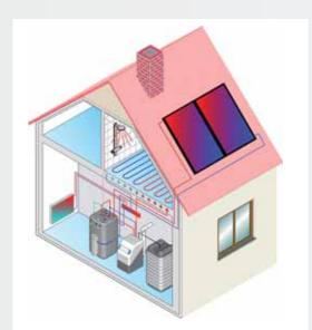
Connection drawing for the ROTEX Solaris System for hot water preparation with heating support: with ROTEX A1 Oil condensing boiler
