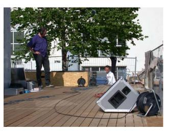
Pictures: Measurement of sound insulation
