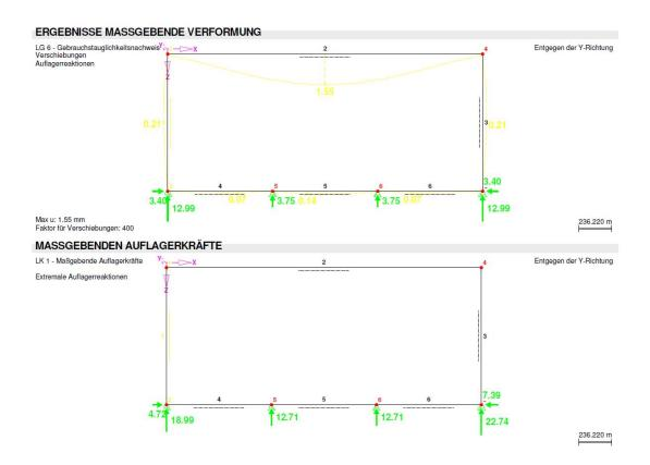
Figure 12: RSTAB-printout, page 8 – critical deformation and bearing reaction
