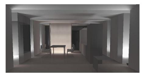
Figure 11: Simulation with Dialux of the iartiticial light of the contest lighting
