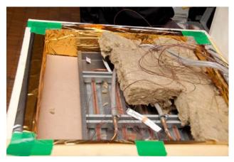
Figure 2.18: Mock-up of the ceiling
