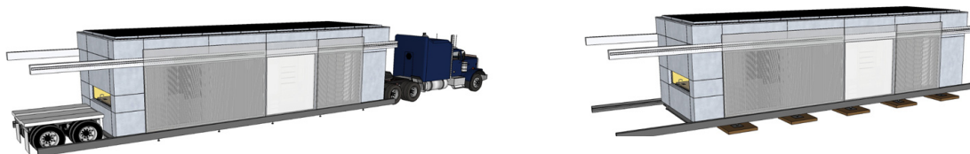
Transport System showing rear wheel bogey assembly and gooseneck and house on temporary foundations
